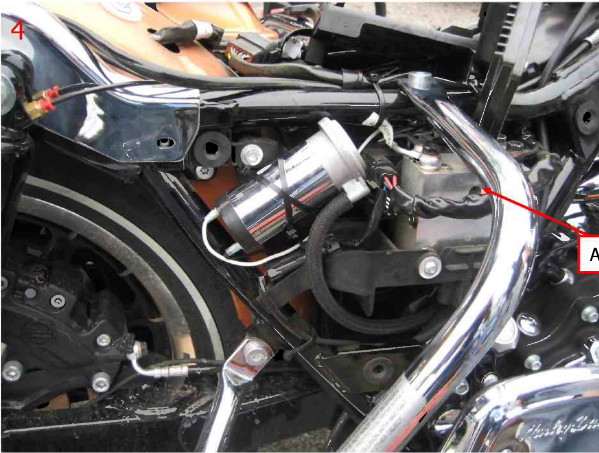
Photo (4) shows the best location for 2008 FLH models with or without ABS with the compressor mounted under the right side cover.
